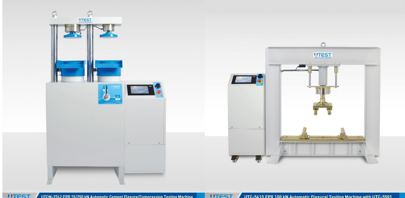
UTEST UTCM-3742.FPR 15/250 kN Automatic Cement Flexure/Compression Testing Machine
